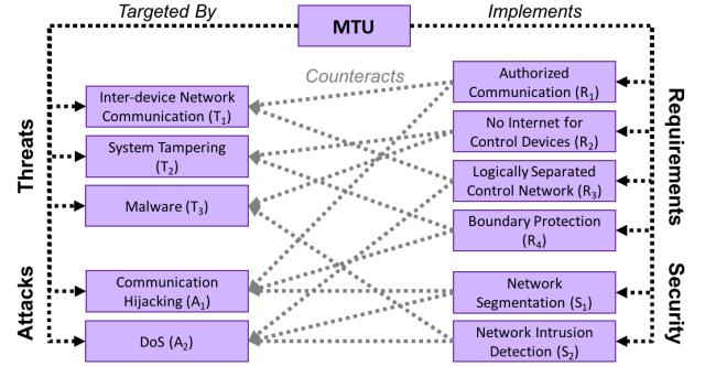
Figure 1: Example Risk Projection featuring the Threats ( $T_n$ ), Attacks ( $A_n$ ), Requirements ( $R_n$ ), and Security Techniques ( $S_n$ ) applicable to an MTU asset.
