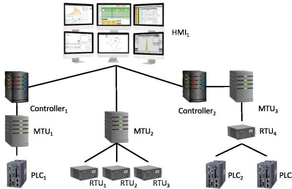
Figure 2: A System Template depicting our running example, developed using Risk Projections based on NIST 800-82 [8].
